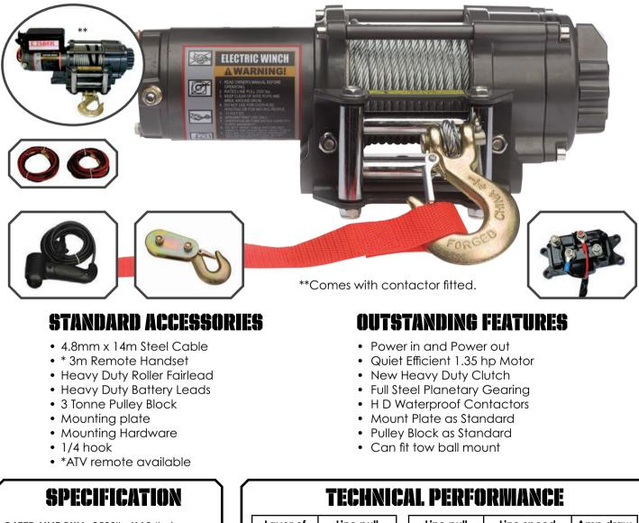
**RATED LINE PULL:** 2500lbs(1134kg) **MOTOR:** 12v : 1.35hp / 0.95kw **GEARING:** 170:1 **BRAKING ACTION:** Dynamic **DRUM SIZE Dia x L:** 37 x 80mm **CABLE Dia x L:** 4.8mm x 14mm **MOUNTING PATTERN:** 79.5mm **DIMENSIONS:** 335 x 113 x 165mm **WEIGHT:** 9kg
